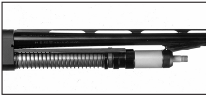
A single-strand recoil spring around the magazine tube returns the bolt to battery. Its movement is in line with the axis of the bore, further contributing to in-line recoil.
